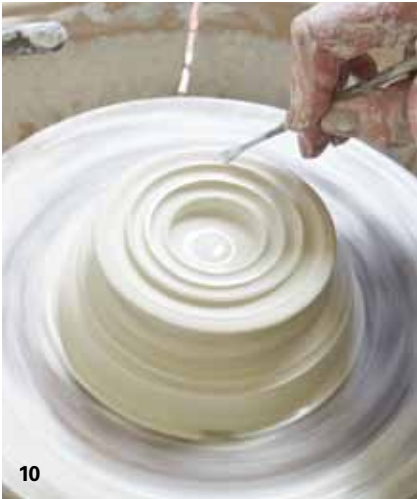
Use a round ended sculptor's tool to create a ring with wider grooves.
