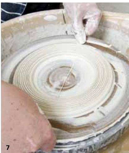
7 Cut a section from the ring with a wire tool held taut against the bat.
