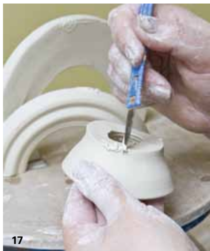
Thoroughly score each surface before joining, the same way as you would join a handle to a mug or jug.
