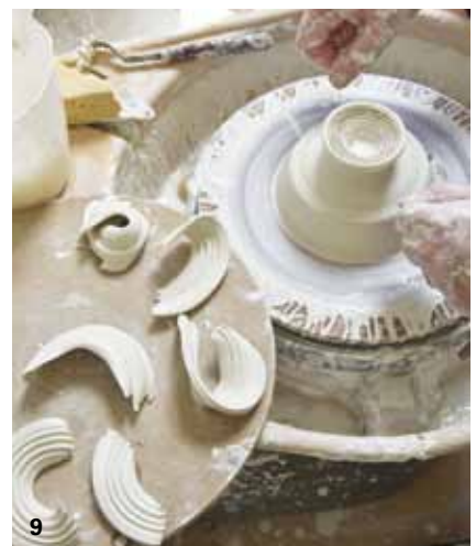
9 Cut off the top of the ring as a complete round piece, and set aside to firm up.
