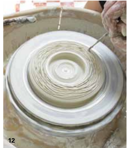
Use a sharp tool to create a criss-crossed surface of thin lines as the wheel spins.
