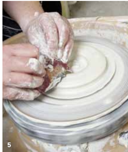
5 Use a flexible, grooved rib (or notched credit card) to contour a thrown ring.
